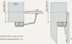
In case the gate leaf is longer than 2.5 m, we recomend the use of an electric lock to apply to the F1000 and F1024. The same application is indispensable in case of the F1100 model.
